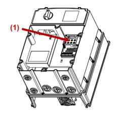
■ Remove the Keypad Case(1) and it's connection cable first, then unfasten a screw(2) from Keypad.
