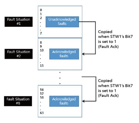
In the diagram, the current Fault Message is saved at Fault Situation #1. Each fault message is saved based on the time of occurrence, from index 0 to 63.
