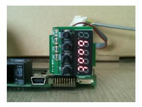
Figure 43 - Ready-state Loader display
