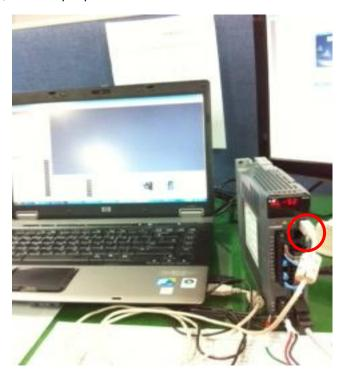
Figure 9 - Installation of USB device driver: Connect the cable
